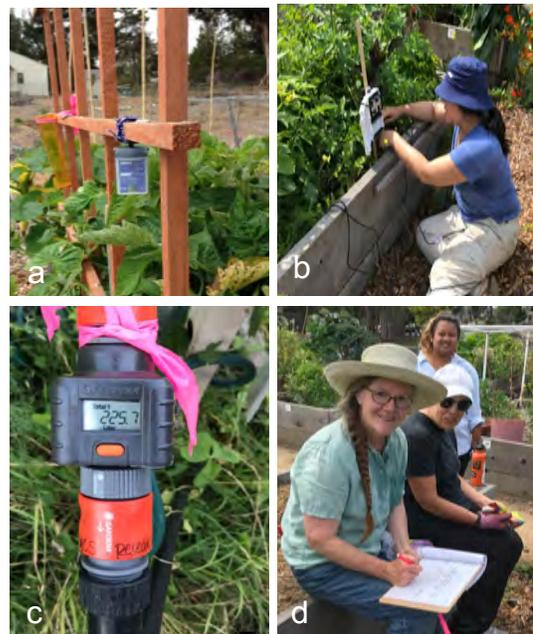
**Fig. 6.** Water-metering study. a) temperature logger, b) Brenda Lin hooking up the soil moisture sensor equipment, c) water meter used in the experiment, d) gardeners filling out the data sheets.
